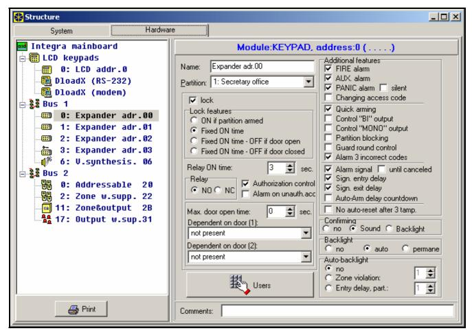
Figure 2. DLOADX program window with partition keypad options.
